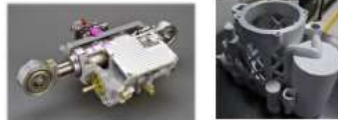
Hydraulic Flight Control Actuator & Additive Manufactured Manifold
